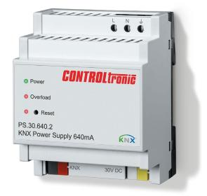
KNX power supply with integrated choke. LEDs for power, overload and reset. Button for automatic reset on the KNX line. Additional auxiliary voltage output with 30V DC. Nominal current at the short-circuit proof outputs is 640mA.
